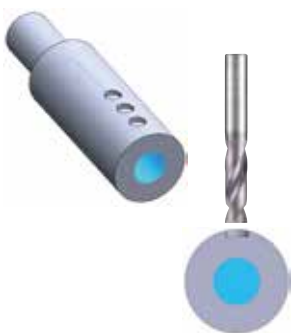
TLDMでガイド穴あけ加工 (円筒面) Guide drilling on cylindrical surface with TLDM
